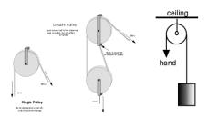
lowered by a pulley. Sometimes a number of pulleys are used to move objects. People use groups of pulleys to move heavy loads, such as boats, pianos, and safes. The more ropes used to hold the load, the stronger the force acting on the load.
