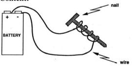
An electric current moving through a wire causes a magnetic field around the wire. If the wire is shaped into loops, the magnetic field gets stronger. An electric current running through a loop of wire makes an **electromagnet**. If the electric current is shut off, the electromagnet is no longer magnetic. The electromagnet is turned off.
